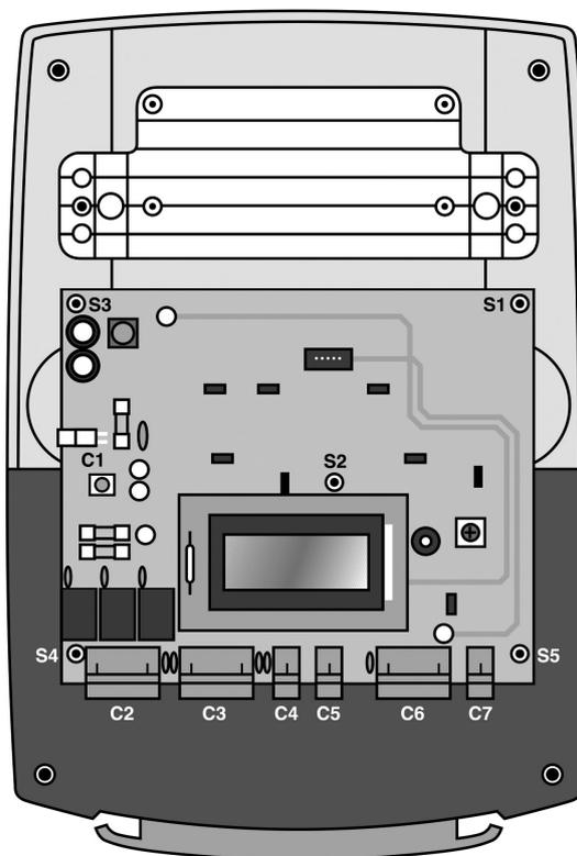
**STEP 5:** To replace the PC Board, align the four spade connectors in the middle of the PC Board using the guide tabs, and gently press the PCB down into place.
