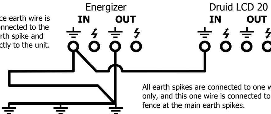
All earth spikes are connected to one wire of the fence only, and this one wire is connected to the rest of the fence at the main earth spikes.
