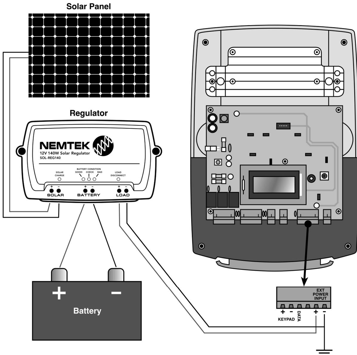
Note: If the Druid LCD 20 has a Nemlink Ethernet card installed, a separate earth spike, not connected to the fence ground, must be installed at least 2m away from the fence earth.
