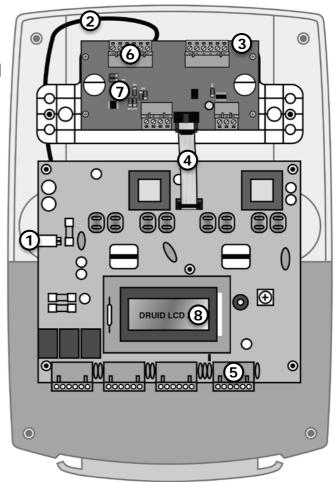
f. Connect the GND, A and B wires going to the next RS485 network device to the DATA OUT GND (marked G), A and B terminals of the RS458 board. [6]
