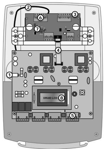
f. Connect the A and B wires coming from the DATA IN of the FG7 to the DATA OUT A and B terminals of the RS485 board. It is not necessary to connect the GND terminals in this step. [6]
