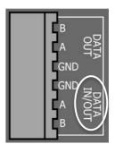
g. Connect the GND, A and B wires going to the next RS485 network device to the DATA OUT GND, A and B terminals of the relay board. [6]
