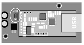
**8-Way Relay Board and 8-Way Smart IO Board JP3**Ensure jumper installed on the 2 upper pins as in the figure
