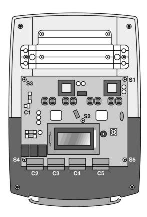
**STEP 5:** To replace the PC Board, first align the box connector near the bottom of the PC Board and then align the four spade connectors at the top of the PC Board using the guide tabs, and gently press the PCB down into place.
