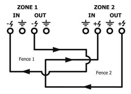
Earth wire connection with no earth loop monitoring
