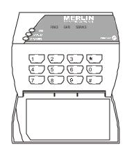
When using only one keypad on an energizer, the installer does not have to concern himself with the actual keypad address. The default address is 1.
