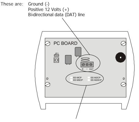
The keypads referred to are distinguishable by the markings 'EE-MCP, EE-M2CP, EE-M9CP and EE-M20CP on the PC board, below the terminal connector.
